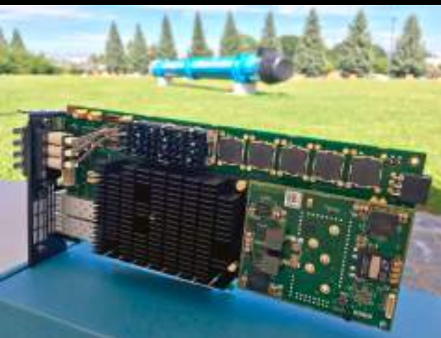
common readout unit (world's largest FPGA)
